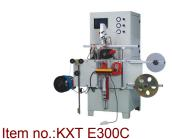
Automatic Winding Machine For Spiral Wound Gasket Product number:KXT E300C
